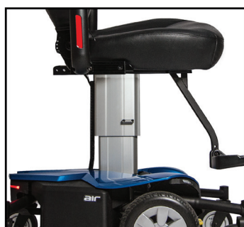
10" Seat lift, which can be operated at 3.5 Mph
